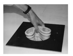
The advanced Amerair design uses nozzle mounted pulse tubes eliminating the need for a venturi at the top of the bag while allowing for efficient pulse cleaning with the pulse of compressed air centered in the bag. Cleaning is further enhanced by balancing the cleaning force coming from each of the pulse tube's orifices by custom varying the diameter of each orifice progressively along the pulse tube.
