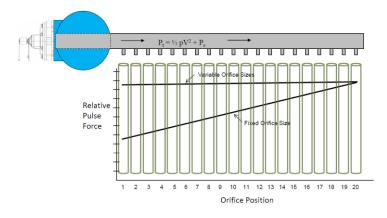
Compartment flow management is critical to successful operation with respect to; pressure drop, bag life, and cleaning performance. Amerair makes use of high and low side flow baffles designed by CFD analysis for balanced compartment flow.
